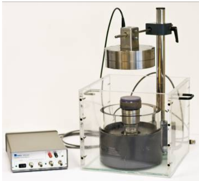
Short Tank immersed in a larger tank to accommodate large transducers
