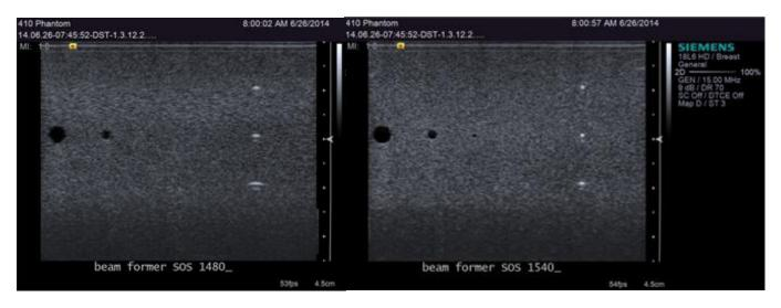
Adjust the gain control to the lowest noise level. This is the point at which you eliminate noise in the anechoic cyst (lower the gain until it just disappears). Record this gain setting and use it for future grey scale measurements. Freeze the image and visually evaluate the grey scale targets. Match each target with a step on the grey bar in the image. Make a hard copy and
