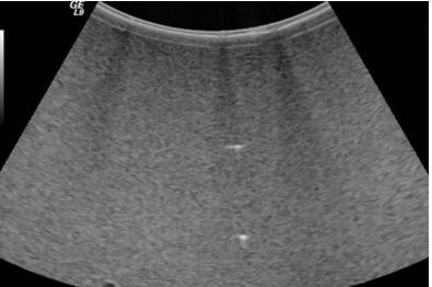
5. Scan the vertical pin targets and freeze the image. Use the electronic calipers to measure the distance between two of the vertical pin targets. Repeat for two of the horizontal pin targets. The vertical pins have 1, 2 or 4 cm spacing while the horizontal pins have 2 or 4 cm spacing.
