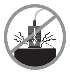
Caution: Do not press the transducer into the scanning surface.
